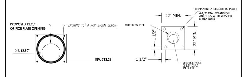
PLATE RESTRICTOR DETAIL: ELEVATION ANCHOR EMBEDMENT SHALL BE 3" MIN.
